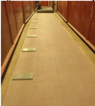
Pigs are walked in a continuous closed loop across the pressure mat (4.3 m with 13,824 sensors) to acclimate the animals to the desired speed and pattern of movement
