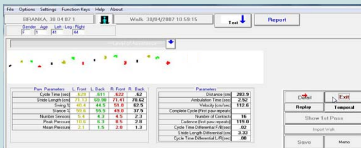
Figure 2 : Screen print from the GAITfour® software after data acquisition and treatment. Footprints had been identified as : Yellow: left forelimb Red: right forelimb Green: left hindlimb Black: right hindlimb
