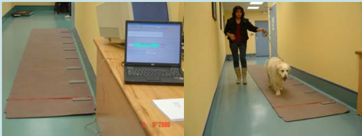
Figure 1 : GAITrite® pressure walkway gait analysis system in situ for dogs
